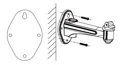
Figure 2-5 Drill Template & Install Mount
