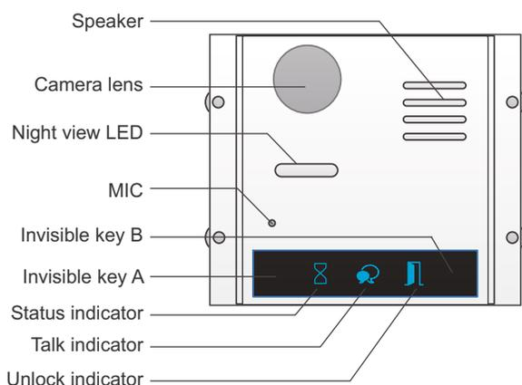
**Note:** Key A and key B can not be seen on the panel, they are cryptic. Normally, key A and key B are not activated. **To activate the buttons, just set the DIP6 to ON.**
