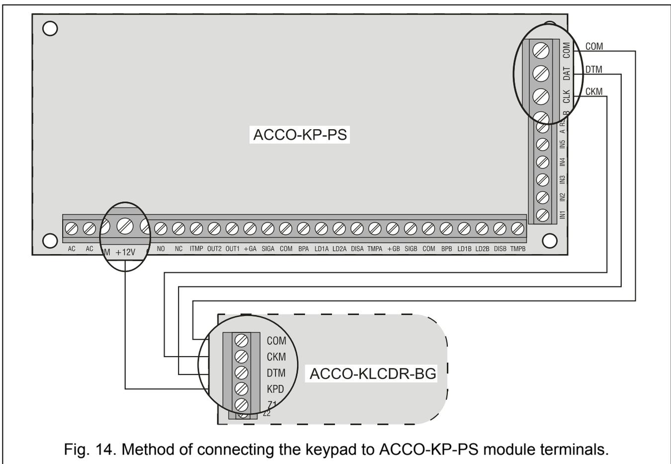
Fig. 14. Method of connecting the keypad to ACCO-KP-PS module terminals.
