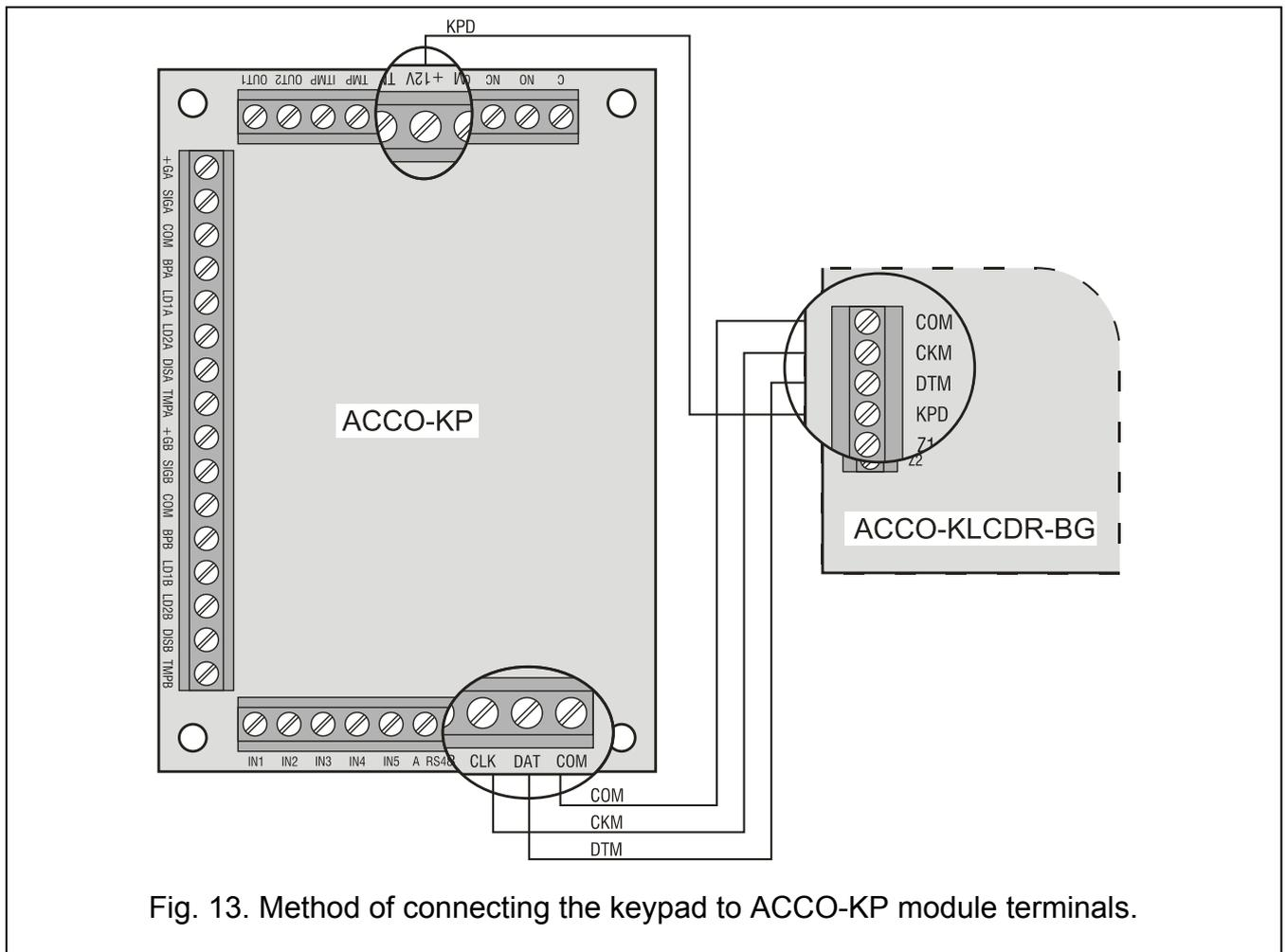
Fig. 13. Method of connecting the keypad to ACCO-KP module terminals.
