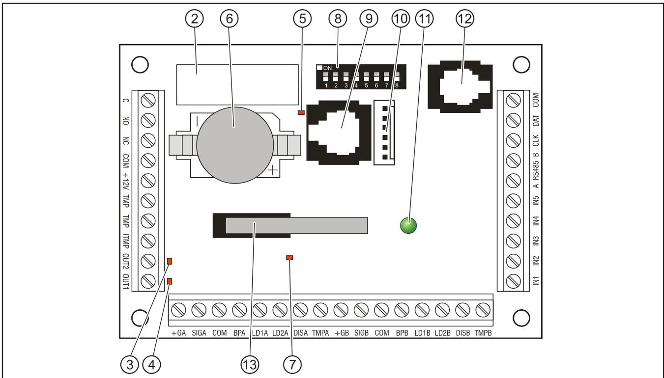
Fig. 2. Schematic view of electronics board in ACCO-KP door controller module.
