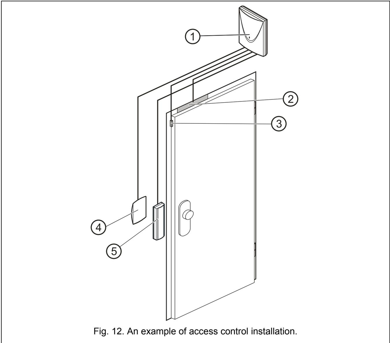
Fig. 12. An example of access control installation.
