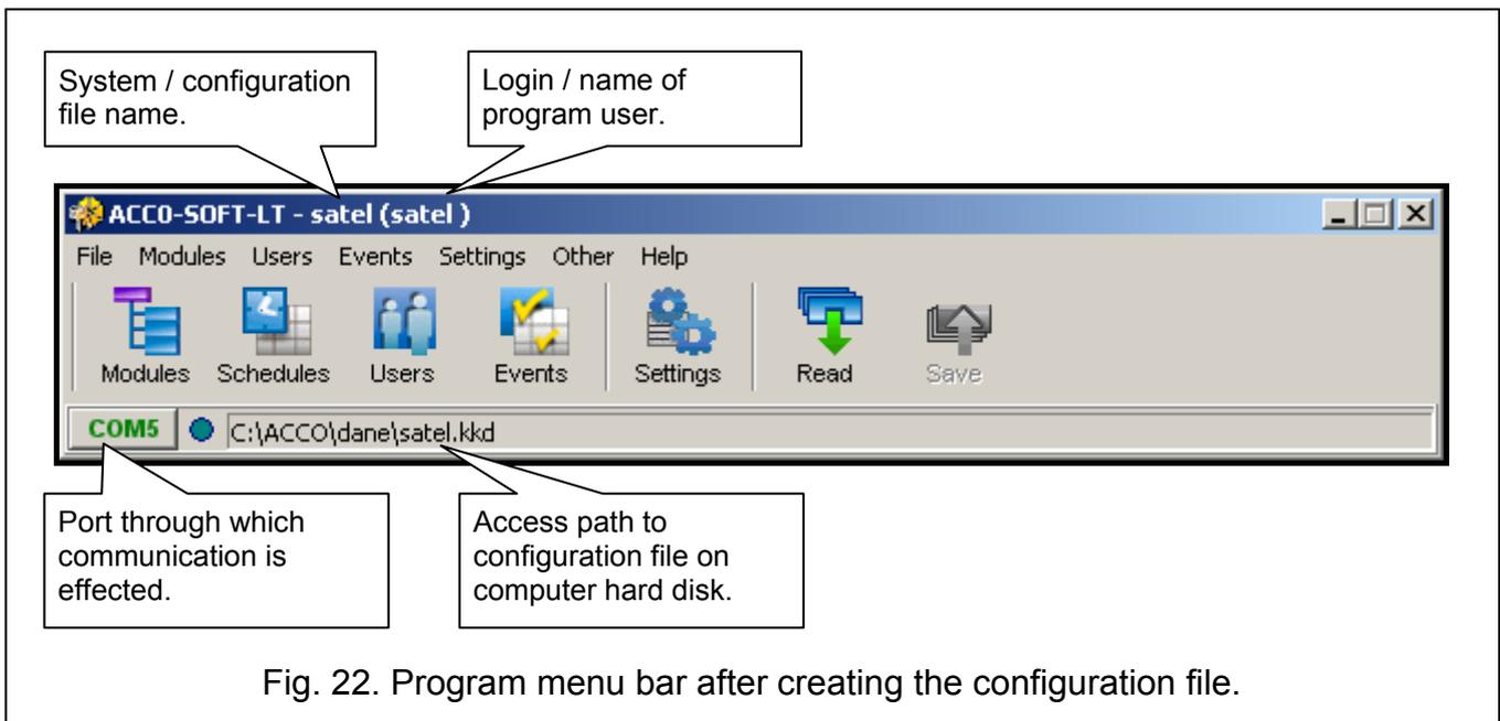
Fig. 22. Program menu bar after creating the configuration file.
