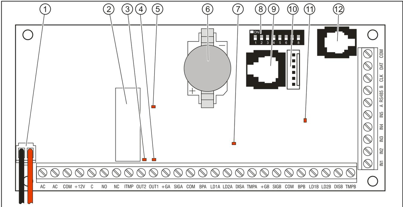
Fig. 1. Schematic view of electronics board in ACCO-KP-PS door controller module.
