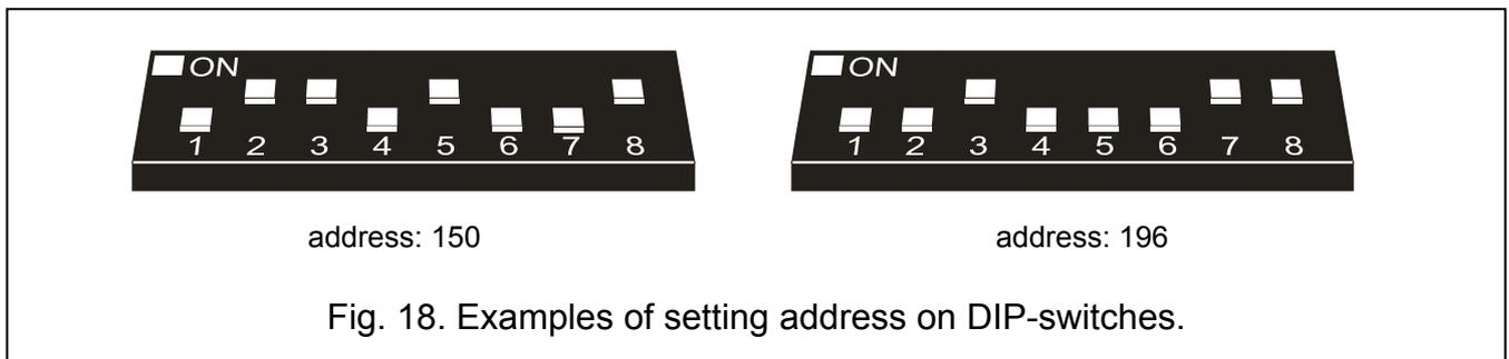
Fig. 18. Examples of setting address on DIP-switches.
