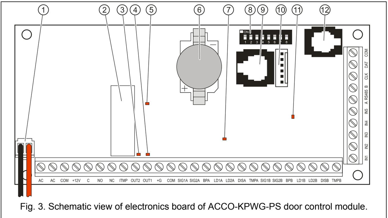
Fig. 3. Schematic view of electronics board of ACCO-KPWG-PS door control module.
