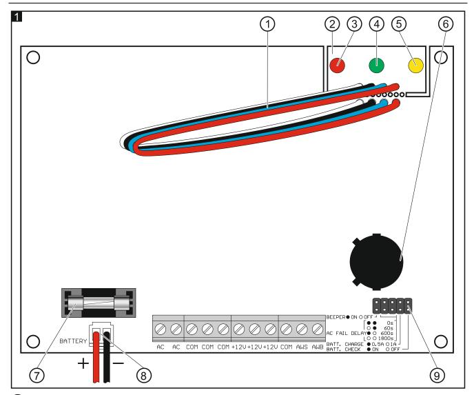
pins for configuring the power supply operating parameters. The symbol on PCB indicates that the jumper is placed across the pins, and the O symbol – that the jumper is removed from the pins.
