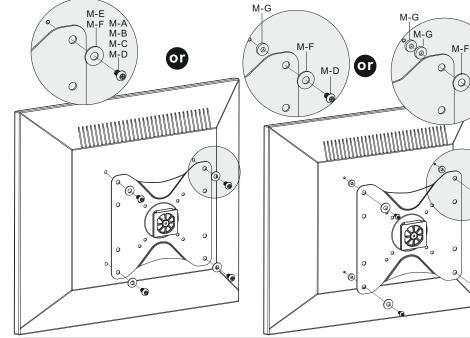
**Note:** Choose appropriate screws, washers and spacers (if necessary) according to the type of screen. Screw VESA plate onto the TV.
