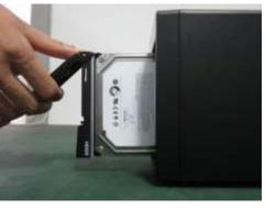
2) Put the HDD to the HDD box at the front.
