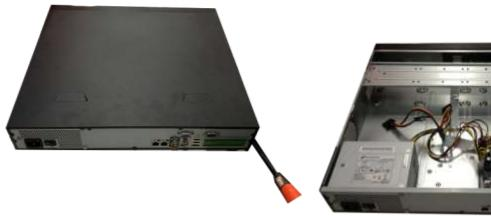
① Use the screwdriver to loose the screws of the rear panel and then remove the front cover.
