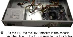
Put the HDD to the HDD bracket in the chassis and then line up the four screws to the four holes in the HDD. Use the screwdriver to fix the screws firmly to secure HDD on the HDD bracket
