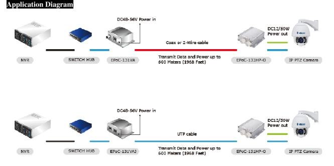
The IP camera and EPOC-131HP cannot receive power through the UTP cable. Please do as below:
