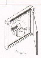
[2] Open the front door by key, pull the door latch downward, refer to the picture, remove the front door from front frame, put them separate for the preparation of the frame assembly.
