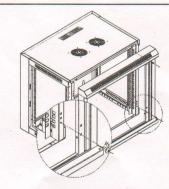
[6] Install front frame by 4pcs of M6\*12 screws (6pcs of M6\*12 screws if more than 18U), refer to the picture.
