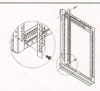
[3] Fix 19" mounting rails to the first holes of top & bottom of side frames by 4sets of M5
