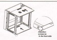
[5] Install top and bottom as shown by the arrow in the picture. Tip: Please note the direction when install bottom, screws will be in the front side,
