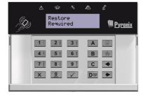
If intelligent arm is enabled by your engineer, the PCX automatically recognises whether to full arm (Arm Mode A), or part arm. (Arm Mode B). 'Flexi'Arm (Page 19) should be disabled for this feature to work properly.
