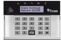
When the time is displayed, enter the number given to you by the ARC. 'Engineer Reset Performed' will be displayed. Press the 🗴 key to back to the time.
