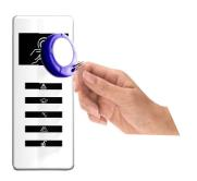
To arm/disarm the PCX system using the external Tag Reader, present a pre-programmed tag to the centre of the prox.
