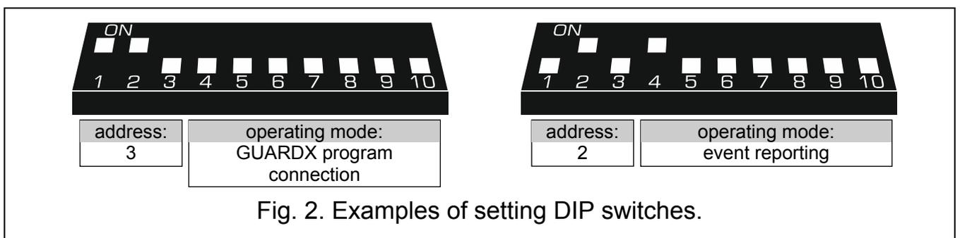
Fig. 2. Examples of setting DIP switches.
