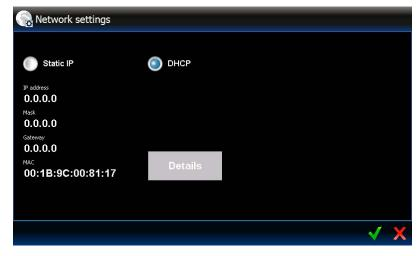
**Static IP** – if this option is enabled, you must program the keypad network settings (tap one of the parameters below and, using the onscreen keyboard that will be displayed, enter the data).
