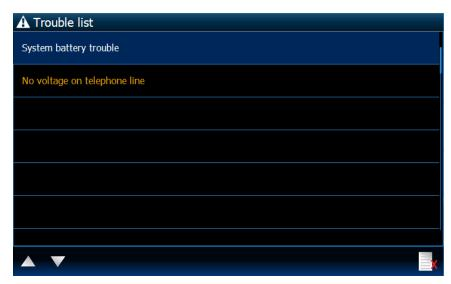
It presents a list of current troubles. The installer can configure the control panel so that the troubles are displayed until cleared by the user. Tap to clear the trouble memory.
