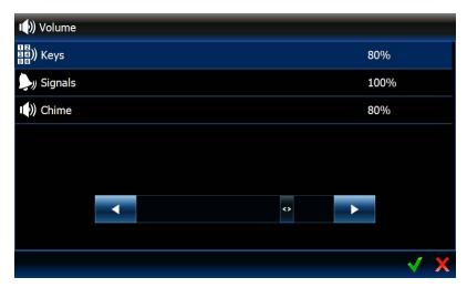
The keypad volume levels may vary, depending on the type of generated sounds. Tap an item in the list to highlight it, and then use the slider to set the volume.
