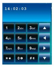
It enables the alarm system to be operated and programmed in the same way as from the LCD keypad with text menu. How such a keypad should be used is described in the control panel programming and user manuals (these manuals are available in electronic form on the www.satel.eu website).
