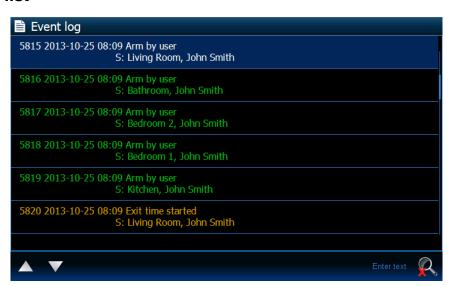
It presents events downloaded from the control panel and saved to the memory card in the keypad. Double tapping an event will display a window with detailed information on the event.
