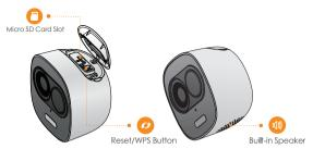
Note: The top cap can be opened with the pry bar from the accessory kit. Press the Reset/WPS Button to enable WPS. Press the Reset/WPS Button for 10 seconds to reset the device.
