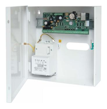
Access control kit for one door. The kit consists of metal enclosure with transformer and networked access controller. The controlled door can be managed on both, read-in and read-out sides, by RS485 (MCT series readers), RACS CLK/DTA (PRT series readers) or Wiegand readers.
