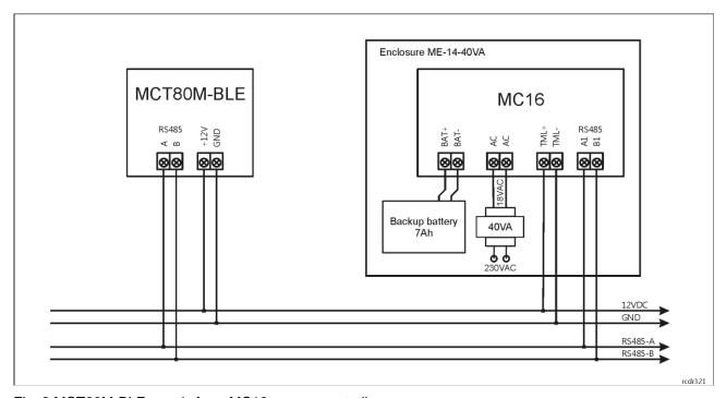
Fig. 2 MCT80M-BLE supply from MC16 access controller
