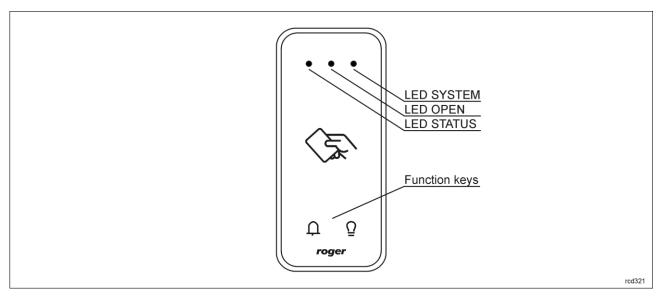
Fig. 3 LED indicators and function keys
