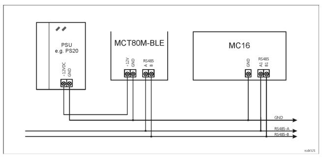
Fig. 1 MCT80M-BLE supply from dedicated power supply unit
