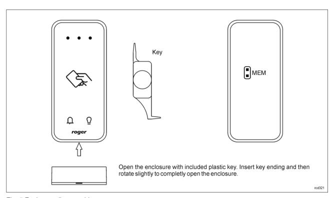
Fig. 5 Enclosure disassembly
