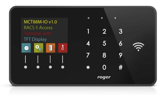
The MCT88M-IO is an access terminal dedicated to RACS 5 system. The terminal is equipped with colour matrix display, sensor type keypad, 4 function keys and MIFARE Ultralight/Classic/DESFire/Plus/NFC/Bluetooth reader. MCT88M-IO can be connected to RS485 bus of MC16 access controller directly or via MCX16-RS expander using Ethernet network (LAN). Alternatively the terminal can be connected to virtual controller through Ethernet network (LAN).
