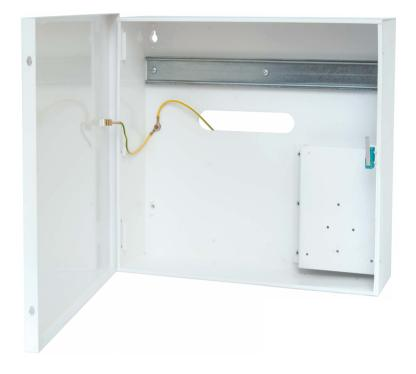
The ME-16 enclosure is dedicated to RACS 5 modules and devices which require installation on DIN rail and 17 Ah battery. The enclosure is equipped with 1 DIN rail and tamper contact. Access to the internal space of the enclosure is protected by a door fixed by screws. The ME-16 is made from a metal sheet painted with a white powder coating.
