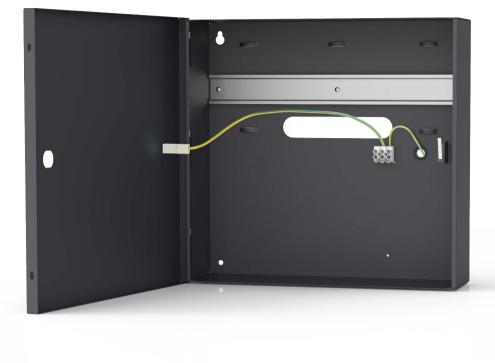
The ME-16 enclosure is dedicated to RACS 5 modules and devices which require installation on DIN rail and 17 Ah battery. The enclosure is equipped with 1 DIN rail and tamper contact. Access to the internal space of the enclosure is protected by a door fixed by screws. The ME-16 is made from a metal sheet painted with a grey powder coating.
