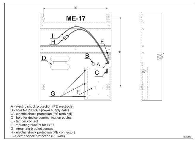
Fig. 1 Arrangement of ME-17 internal components
