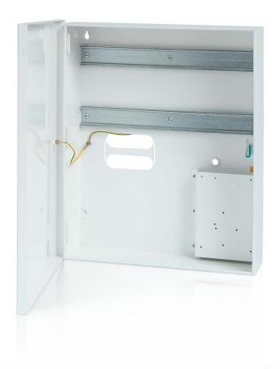
The ME-17 enclosure is dedicated to RACS 5 modules and devices which require installation on DIN rail and 17 Ah battery. The enclosure is equipped with 2 DIN rails and tamper contact. Access to the internal space of the enclosure is protected by a door fixed by screws. The ME-17 is made from a metal sheet painted with a white powder coating.
