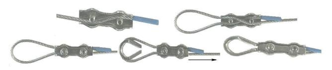
Attach the thimbles and tighten the cable
