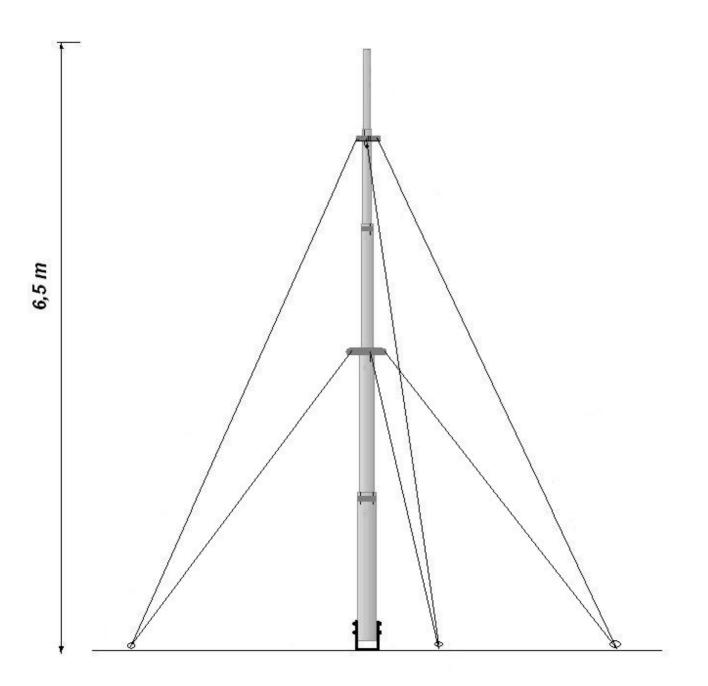
The mast requires periodic inspection of bolted connections and general condition.
