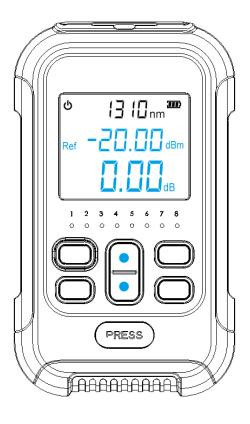
After power on, enter the interface of OPM, press REF to set the current power as the reference power, switch the relative optical power test (insertion losstest) and absolute power test. In the relative power test mode, the insertion loss (dB) and the reference value is displayed simultaneously. Short press "dB" to switch linear power and absolute power display. The units of linear power, absolute power and relative power are W, dBm and dB respectively.
