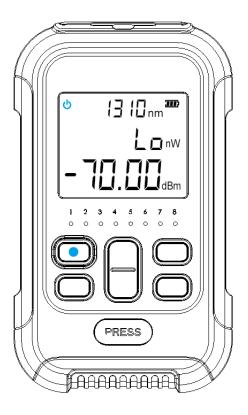
After pressing  $\circlearrowleft$  briefly, the meter will turn on and start the automatic shutdown function. The default automatic shutdown time is 10 minutes. If you want to cancel the function, press and hold the power key for two seconds, and the  $\circlearrowleft$  icon dis appears, the automatic shutdown will be cancelled.
