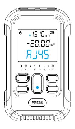
In the test interface of OPM, long press the dB key to display the word "RJ45" on the screen. At this time, enter the RJ45 cable sequence test, connect one end of the network cable to the RJ45 port in the bottom, and connect the other end to the remote tester. Short press the dB key to exit. Long press the dB key again, "=" displays on the upper left corner of the screen, enter the cable tracking mode, and short press the dB key to exit.
