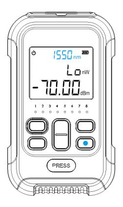
In the interface of OPM, short press the  $\,^{\lambda}$  key to switch the measurement wavelength. Ten different wavelengths can be selected: 1310nm, 1550nm, 1577nm, 1490nm, 1625nm, 1650nm, 850nm, 1270nm, 1300nm and 980nm. In order to ensure the accuracy of the test, the selected wavelength must be consistent with the measured optical signal.
