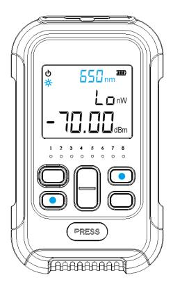
After power on, long press the \*/VFL key to turn on the VFL, short press to flash and turn off.
