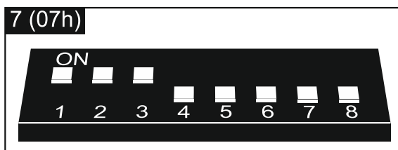
Fig. 6. Setting DIP-switches in the INT-RX-S expansion module.
