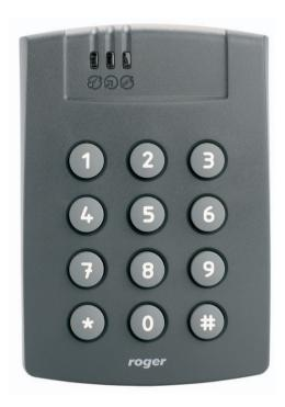
Each PRT64MF series reader can be used as a universal identification point connected to the access controller or configured for autonomous work, as a simple access controller for a single door. In the first case, the reader's functionality is limited only to reading an identi-
