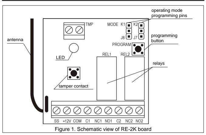
As just one relay is installed on the electronics board of the RE-1 controller, the board has neither the K2 pins or the second relay terminals.
