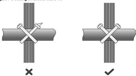
If cables are to be bent, bind them first but do not tie cable ties within the bend to avoid stress on the cables, which may otherwise cause the wires inside to break, as shown in Figure 7-6.
