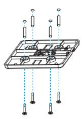
(2) Align the square feet on the rear of the AP with the mounting holes on the bracket.
