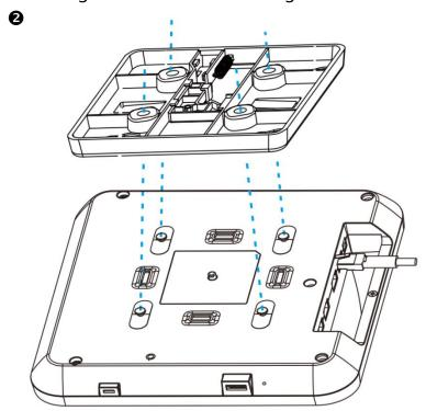
Install the Ethernet cable first before you mount the AP onto the brackets.
