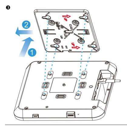
A For ease of cable routing, you can adjust the direction of the AP accordingly.
