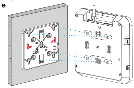
Install the Ethernet cable first before you mount the AP onto the brackets.
