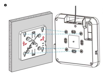
🛕 Install the Ethernet cable first before you mount the AP onto the brackets.
