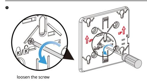
Loosen the screw on the mounting bracket and enable the hidden lock.
