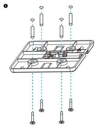
Drill four holes on the ceiling, tap the wall anchors into the holes, and attach the mounting bracket to the wall using the screws.
