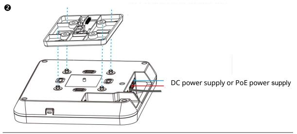
⚠ Install the Ethernet cable first before you mount the AP onto the brackets.
