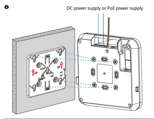
⚠ Install the Ethernet cable first before you mount the AP onto the brackets.
