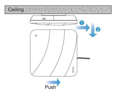
Hold up the two sides of the AP with hands, and attempt to push it in four directions (the AP can be pushed out only in one direction).
