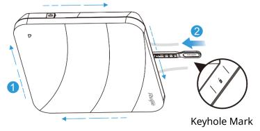
Unlock the hidden lock. If you hear a click sound after the key is inserted into the keyhole and the key cannot be pulled out, the unlocking is successful.
