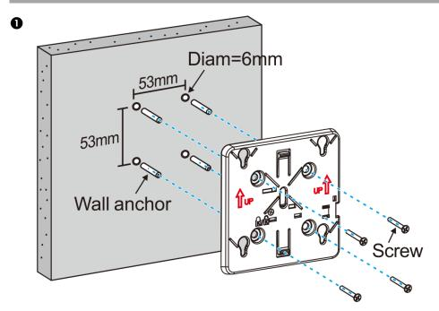
Drill four holes on the wall, insert the anchors into the holes with the arrow on the mounting bracket facing up, and attach the mounting bracket to the wall using screws.
