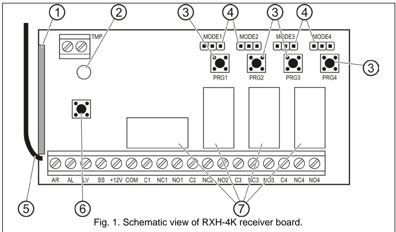
Fig. 1. Schematic view of RXH-4K receiver board.
