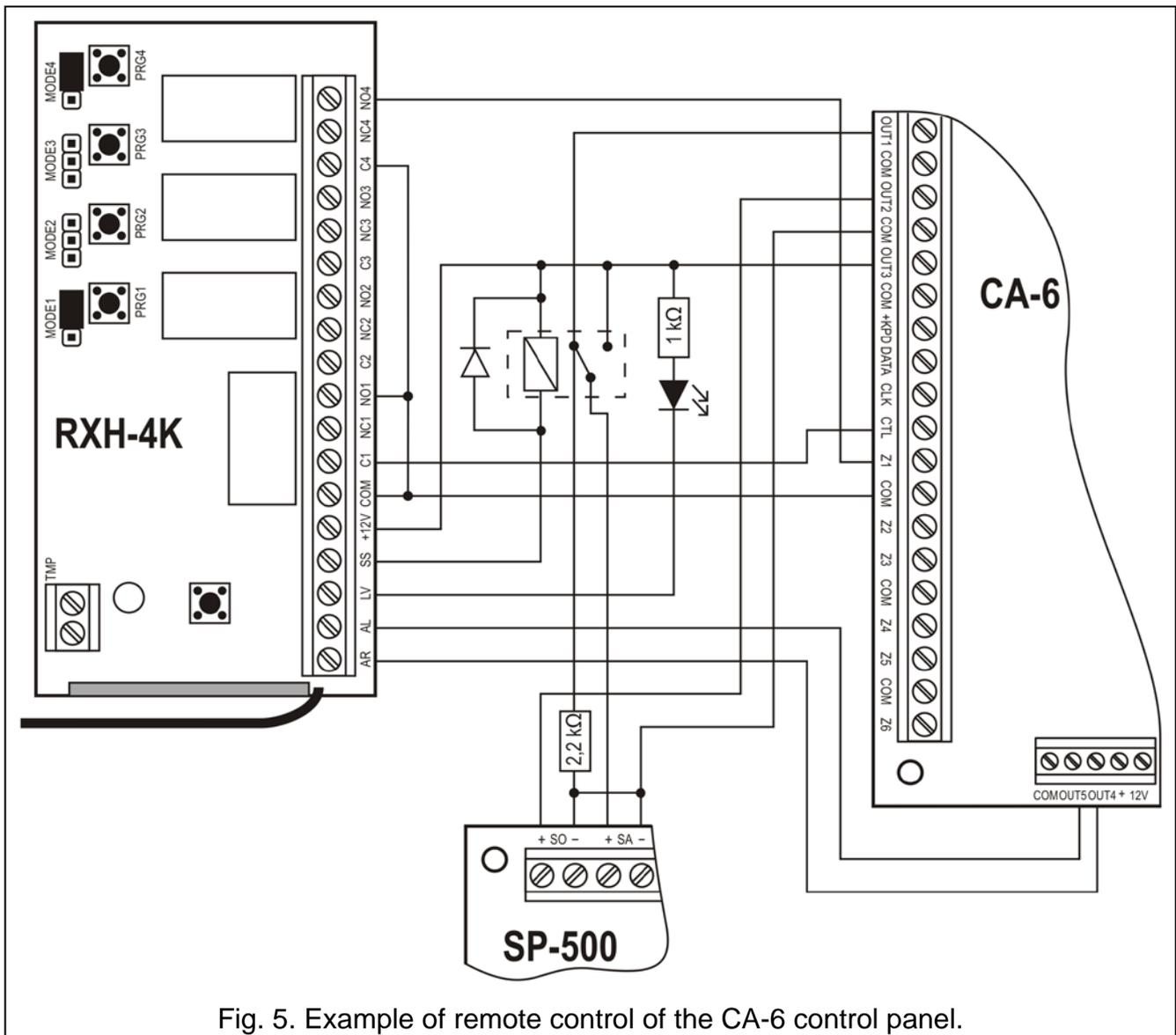
Fig. 5. Example of remote control of the CA-6 control panel.
