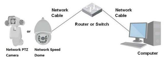
All devices have the same IP address (192.168.1.108 by default) when they are delivered out of factory. To make the Device get access to network smoothly, plan available IP segment reasonably according to practical network environment.
