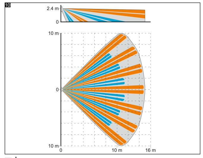
Figure 10 shows the coverage area of the SLIM-PIR detector with a wide-angle lens (WD), which is installed in the detector by default. You can use the enclosure cover
