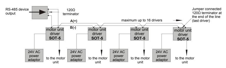
ID number assign, protocol change and 120Ω resistor connection – switchers and jumper configurations:
