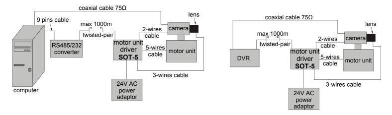
Schematic diagram for many drivers to the one system connection:
