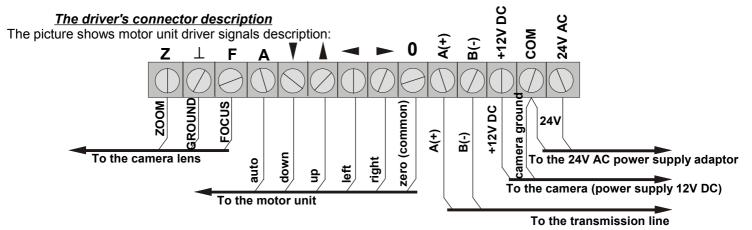
ZOOM - lens zoom control (for 4-wires connections 2 wires have to be join together),
