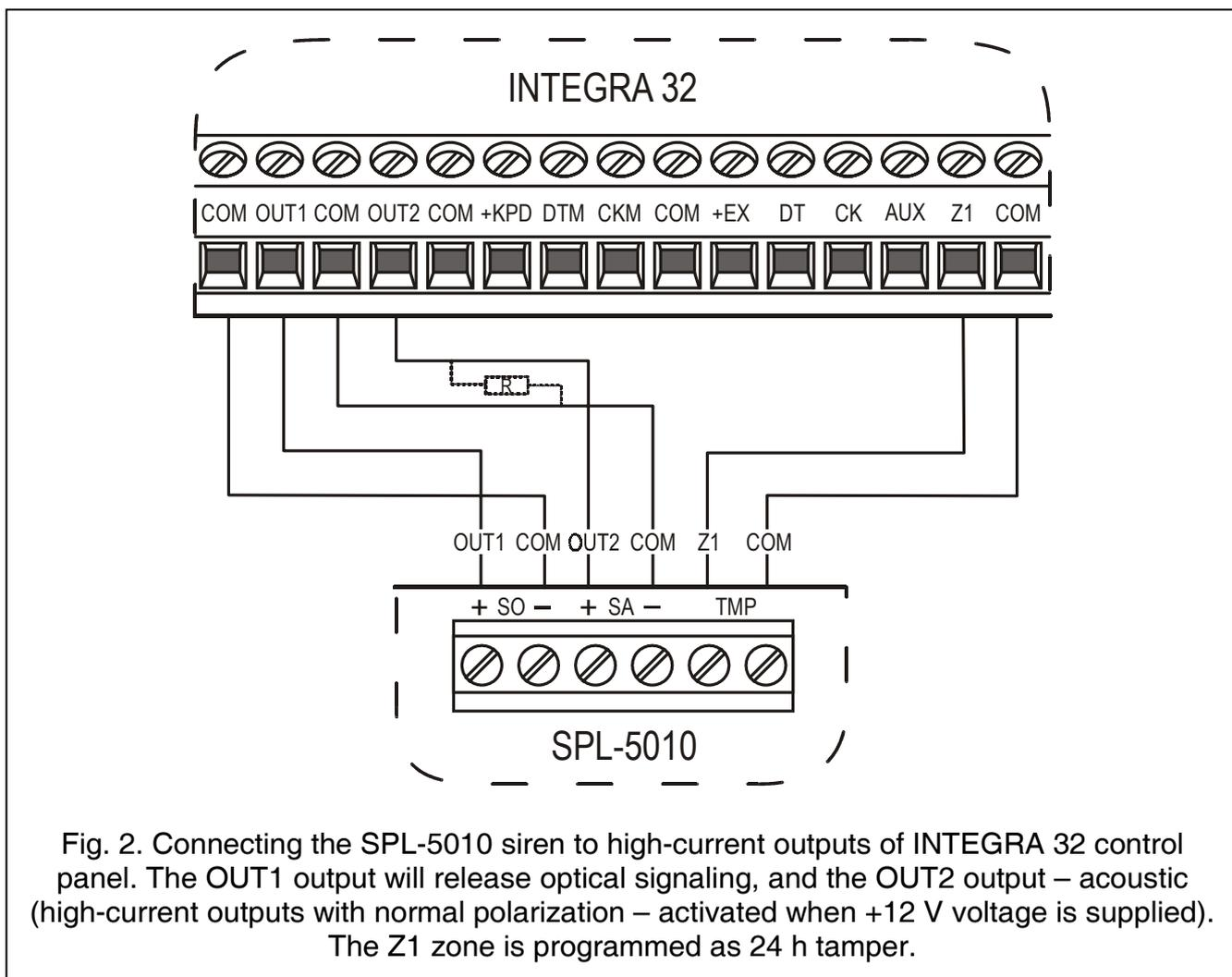
The SPL-5010 siren can be used with any source of alarm signal which in emergency situation generates 12V direct voltage on its alarm output(s) or whose output will be shorted to the common ground (0V). Connecting +12 V power supply to the "+ SA -" terminals will trigger the acoustic signaling, and to the "+ SO -" terminals - the optical signaling in the SPL-5010 device. Choosing the way of signaling activation you need to remember about the maximum control panel outputs load capacity.
