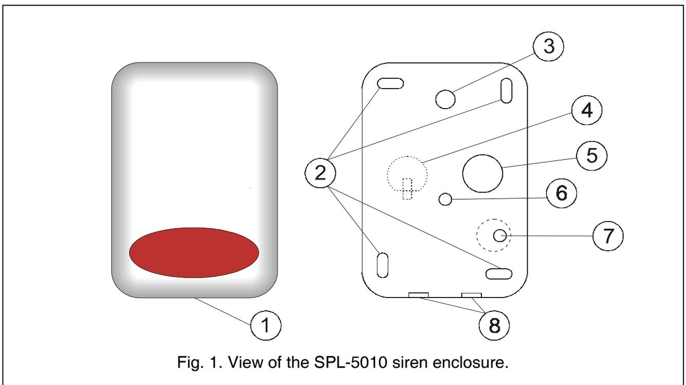
The SPL-5010 siren should be mounted on flat surface, at a place as much inaccessible as possible so that the risk of tampering is minimized. The siren must be attached to the surface by means of screws and expansion plugs. In order to take off the cover, remove the retaining screw and lift it by an angle of approx. 80°.
