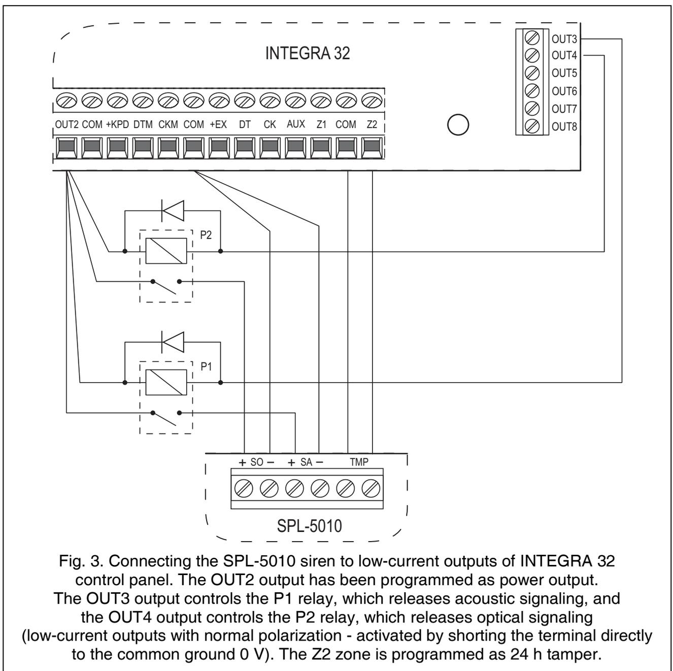
Fig. 3. Connecting the SPL-5010 siren to low-current outputs of INTEGRA 32 control panel. The OUT2 output has been programmed as power output. The OUT3 output controls the P1 relay, which releases acoustic signaling, and the OUT4 output controls the P2 relay, which releases optical signaling (low-current outputs with normal polarization - activated by shorting the terminal directly to the common ground 0 V). The Z2 zone is programmed as 24 h tamper.
