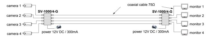
To full protect all devices connected to the line against lightning discharges the above connecting diagram is recommended.
