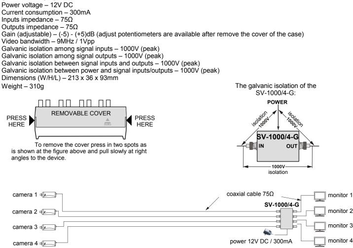
The above schematic diagram allows to eliminate signal disturbances existing due to difference in voltage between camera ground and monitor ground. The voltage results from this difference can adds up to useful signal voltage. It makes low frequency disturbances (e.g. slowly vertical moving black fields).
