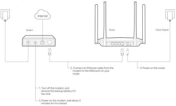
5. Verify that the hardware connection is correct before continuing.
