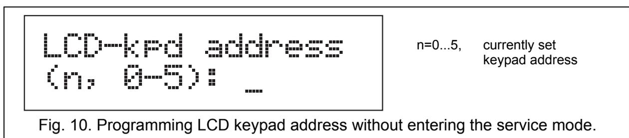
Fig. 10. Programming LCD keypad address without entering the service mode.
