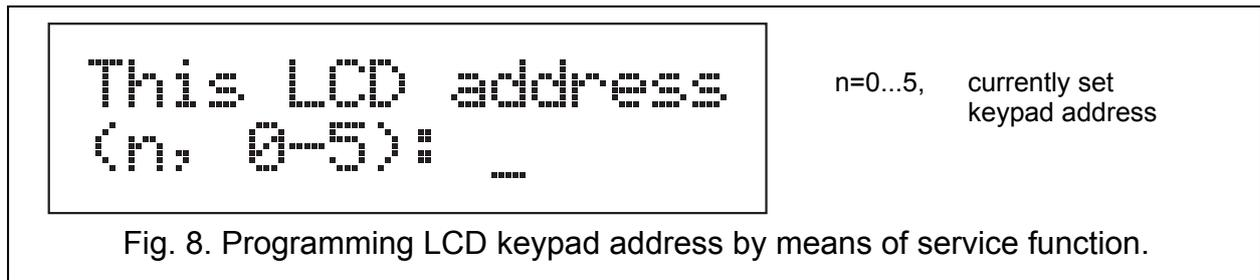
Fig. 8. Programming LCD keypad address by means of service function.
