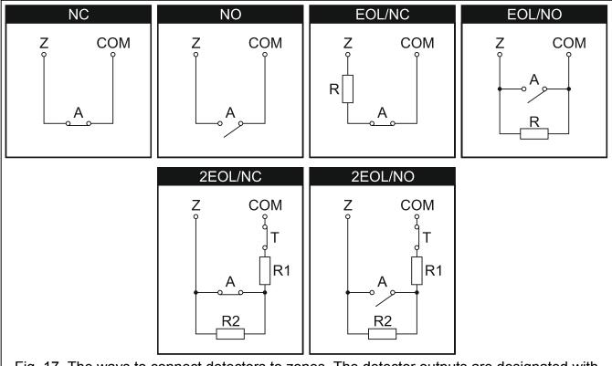
Fig. 17. The ways to connect detectors to zones. The detector outputs are designated with letters: A - alarm, T – tamper. R=R1+R2.
