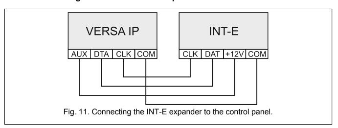
Up to three INT-E / CA-64 E / CA-64 EPS expanders can be connected to the control panel. This enables expansion of the system by adding up to 24 programmable wired zones. Using the expander DIP-switches:
