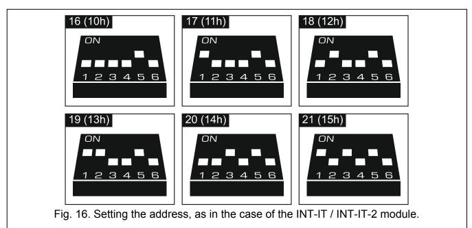
Up to 6 INT-CR / INT-IT / INT-IT-2 devices can be installed in the system. Addresses from the 16 (10h) to 21 (15h) range should be set in the devices.
