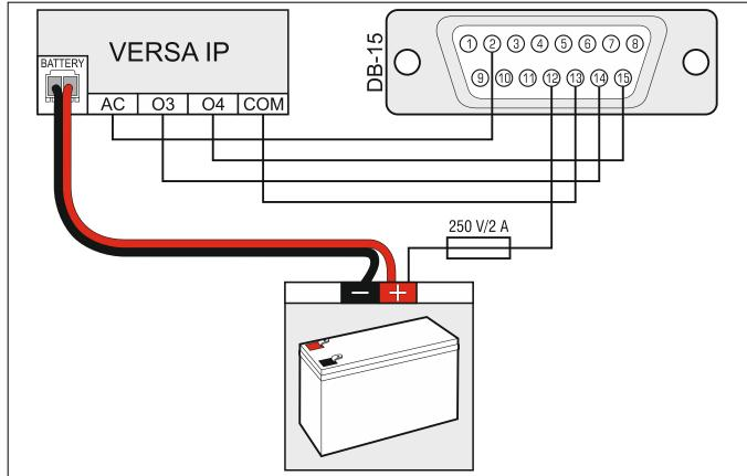
Fig. 19. Connecting the NOKTON NR2-DSC transmitter to the control panel. The DB-15 female connector is shown from the solder side.
