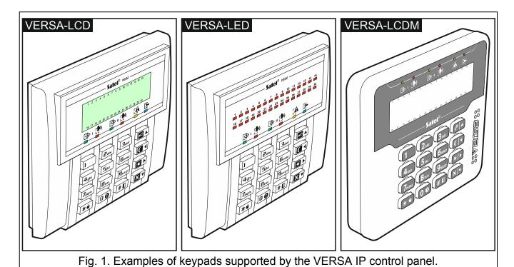
SATEL offers the following keypads for VERSA IP alarm control panels:
