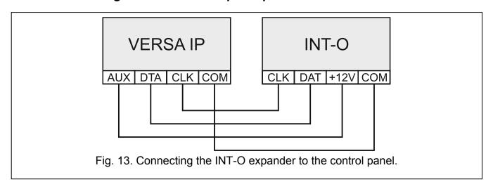
One INT-O / INT-ORS / CA-64 O / CA-64 OPS expander can be connected to the control panel. This enables expansion of the system by adding 8 programmable wired outputs. Address 15 (0Fh) must be set in the expander. In the case of the INT-ORS expander, you must also use the DIP-switches to define how the expander is to be identified (for detailed information please refer to the manual delivered with the expander).
