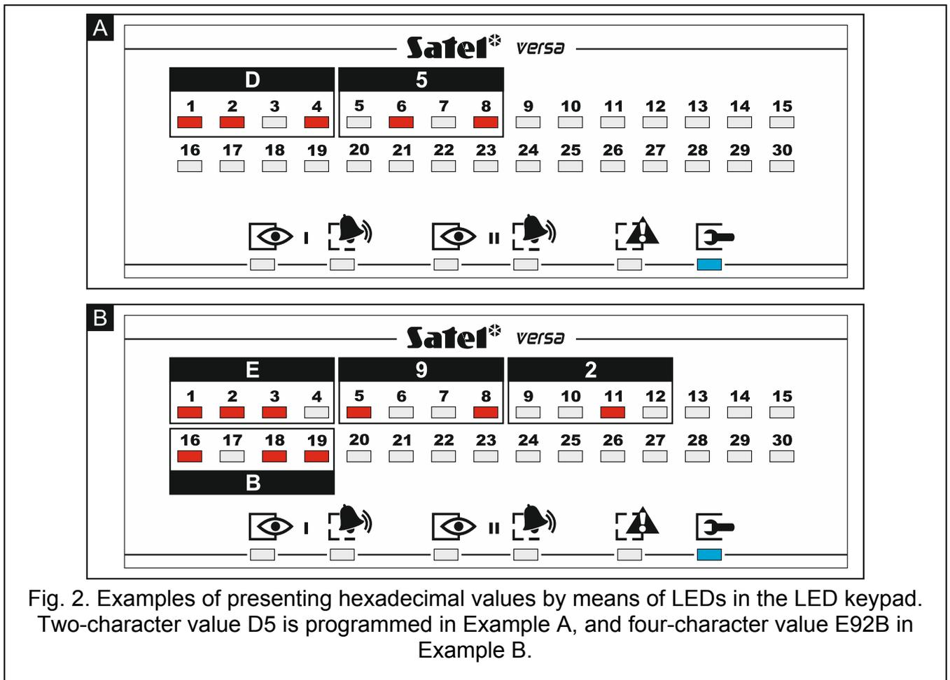
Fig. 2. Examples of presenting hexadecimal values by means of LEDs in the LED keypad. Two-character value D5 is programmed in Example A, and four-character value E92B in Example B.
