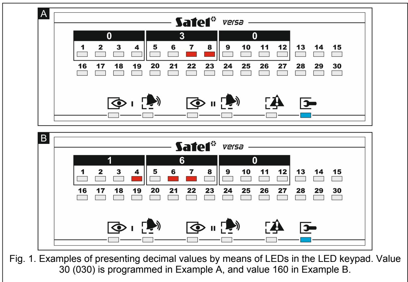
Fig. 1. Examples of presenting decimal values by means of LEDs in the LED keypad. Value 30 (030) is programmed in Example A, and value 160 in Example B.
