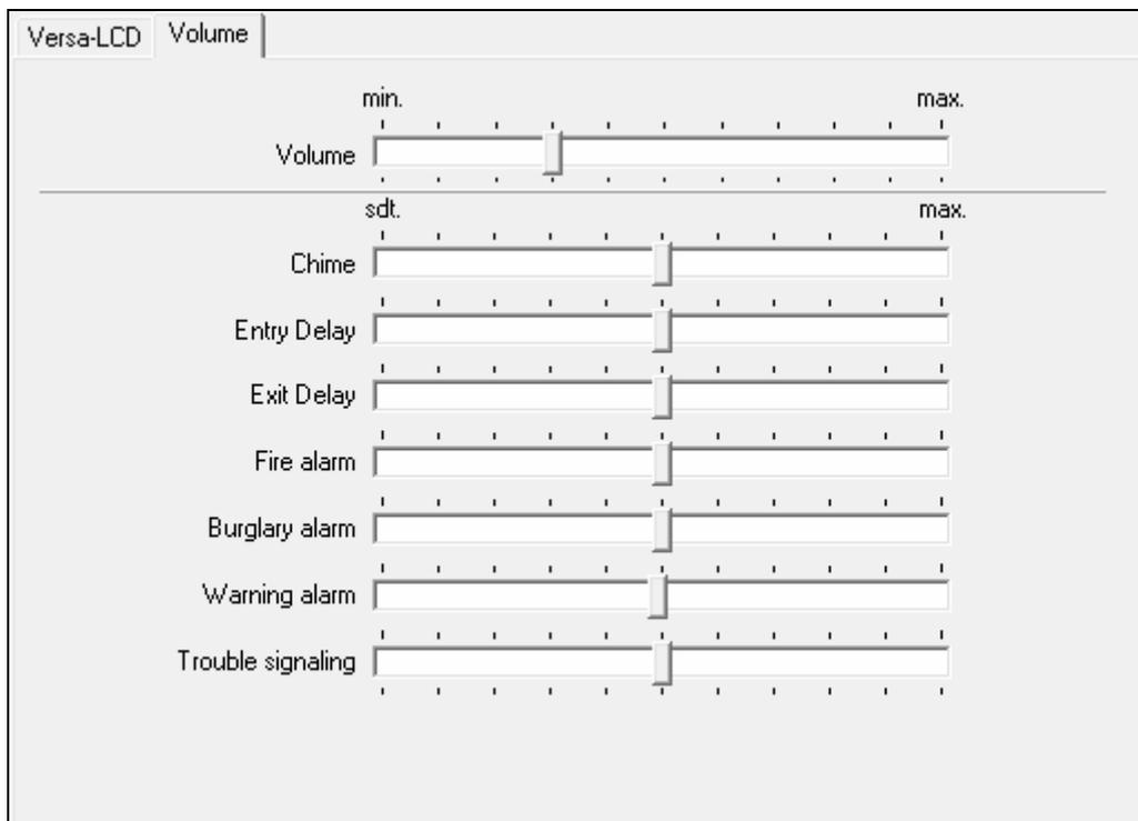
Fig. 17. DLOADX program: configuring the keypad volume.
