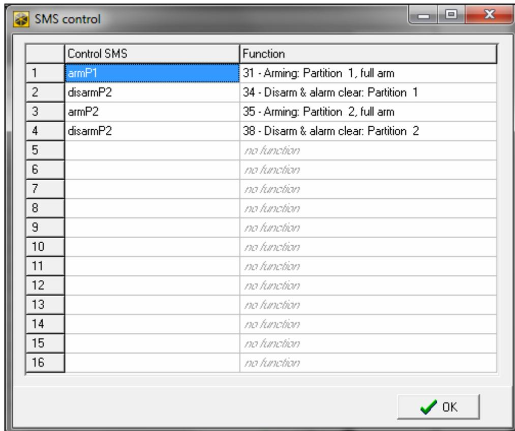
Fig. 30. DLOADX program: “SMS control” window.
