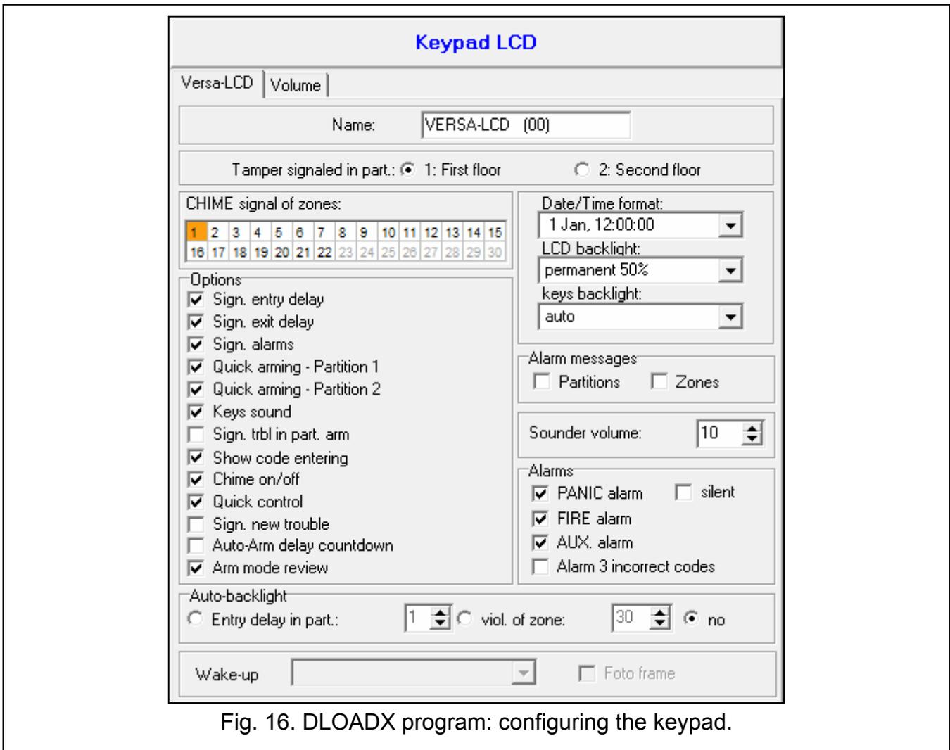
Fig. 16. DLOADX program: configuring the keypad.
