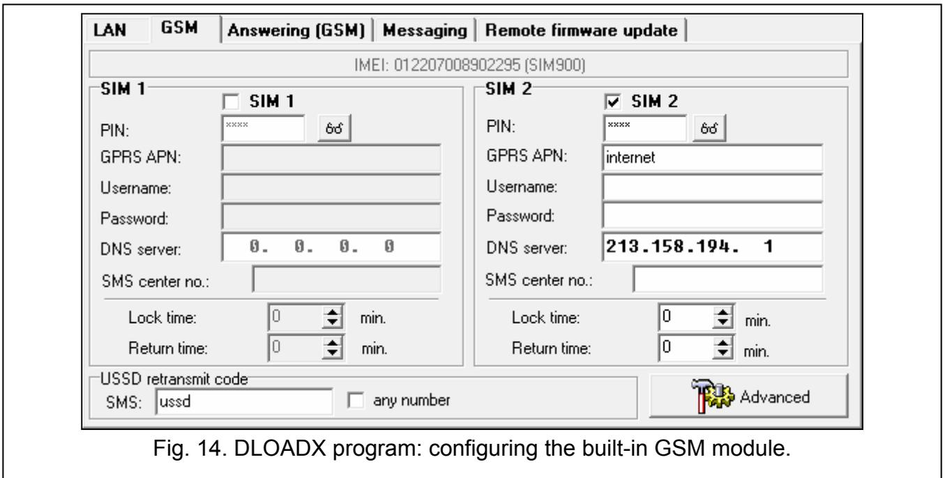
Fig. 14. DLOADX program: configuring the built-in GSM module.
