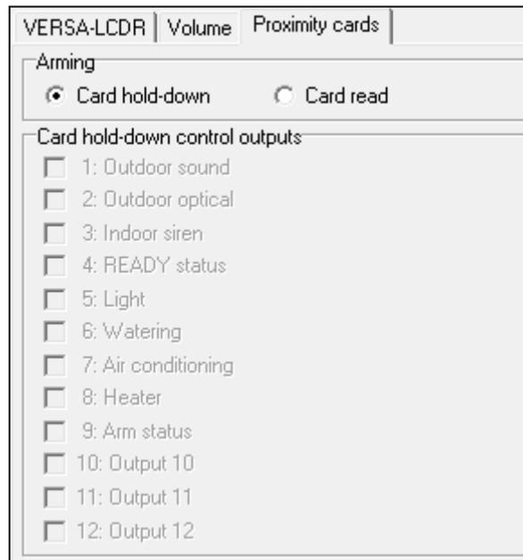
Fig. 18. DLOADX program: configuring operation with proximity cards.
