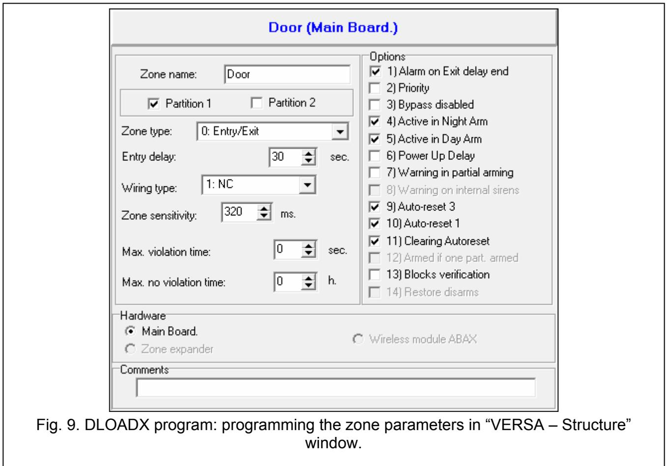
Fig. 9. DLOADX program: programming the zone parameters in “VERSA – Structure” window.
