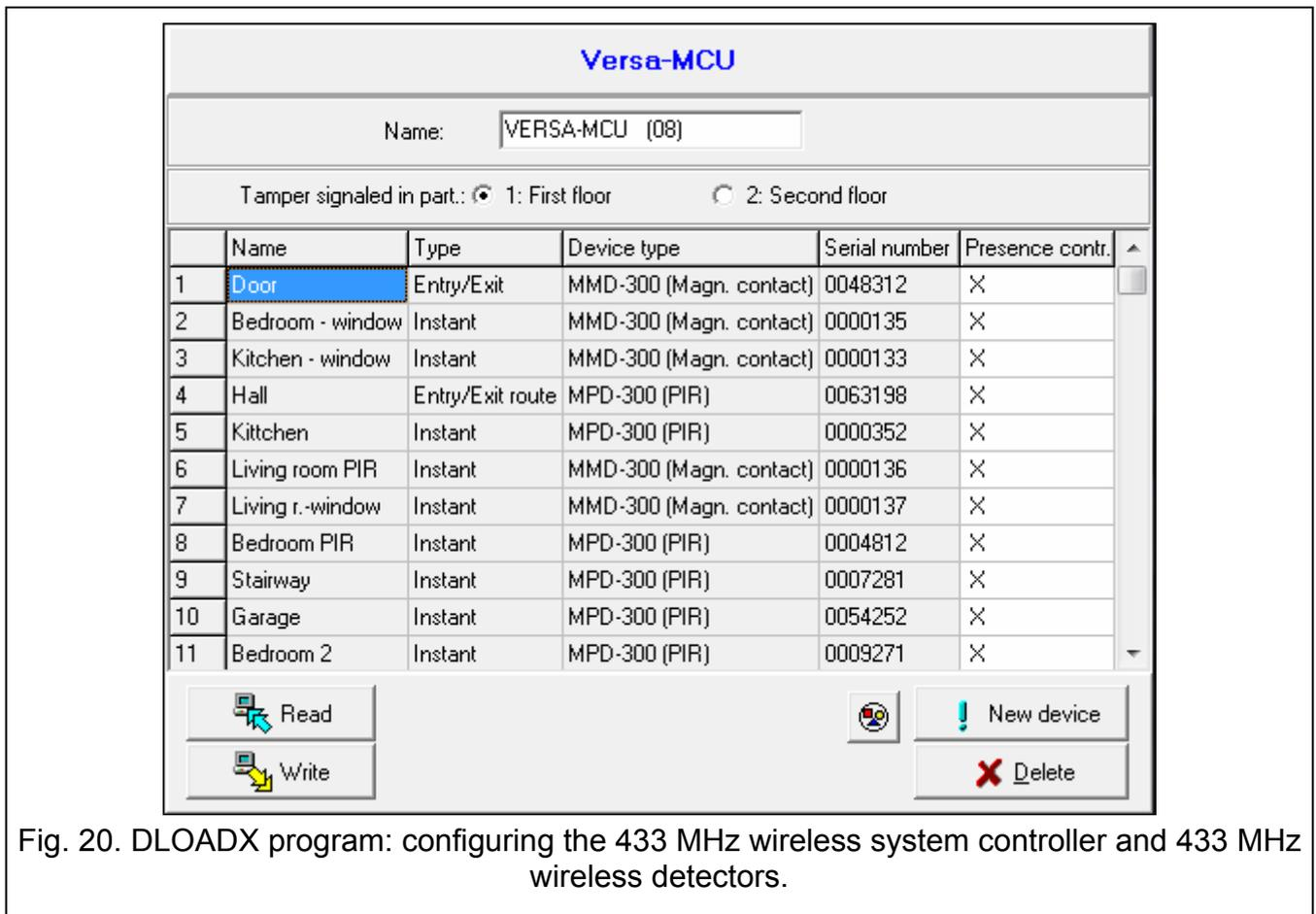
Fig. 20. DLOADX program: configuring the 433 MHz wireless system controller and 433 MHz wireless detectors.
