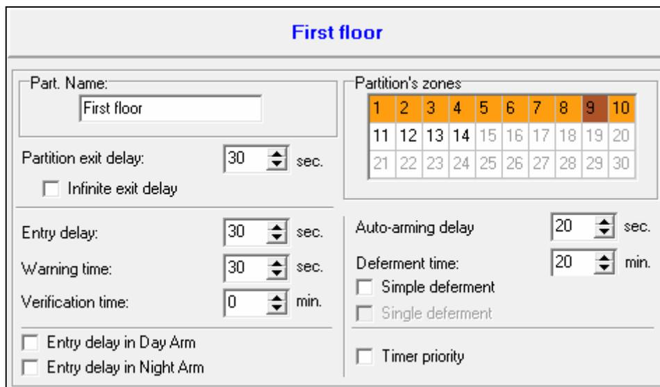
Fig. 7. DLOADX program: configuring partition parameters in the “VERSA – Structure” window.
