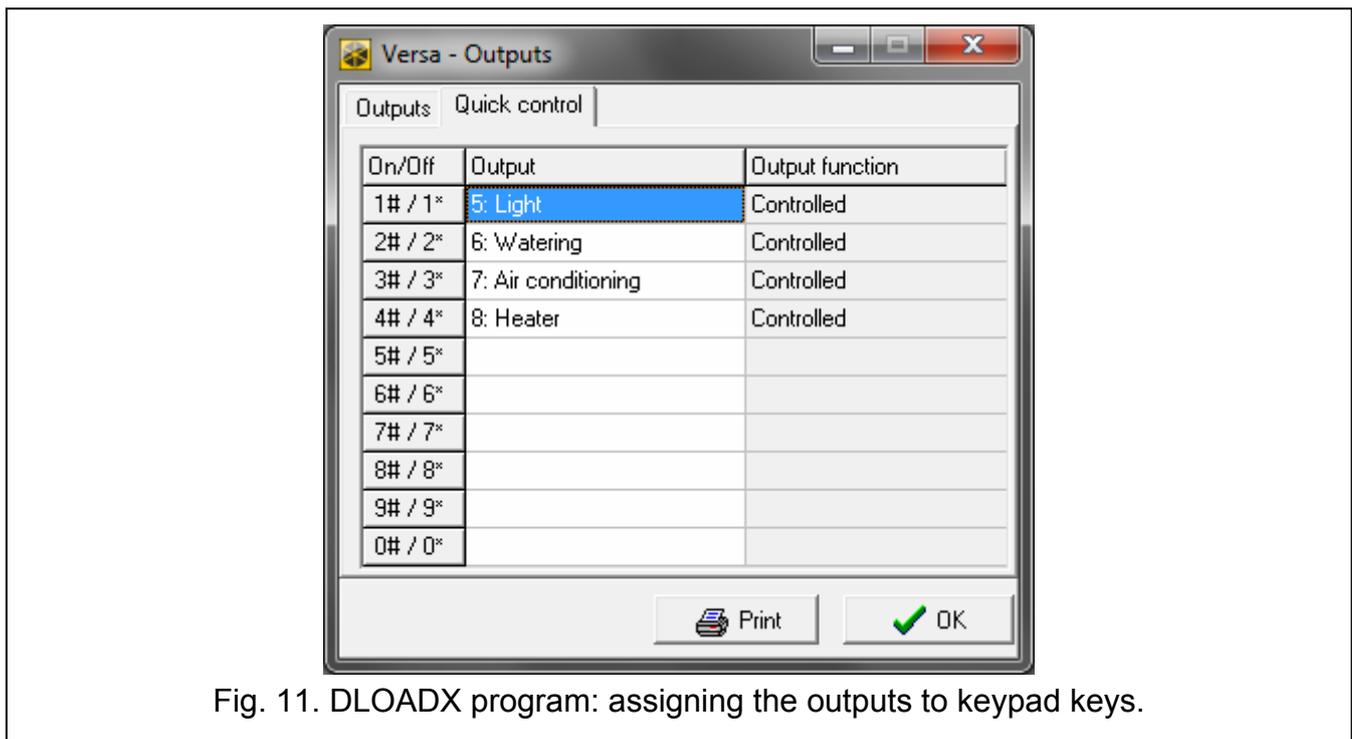
Fig. 11. DLOADX program: assigning the outputs to keypad keys.
