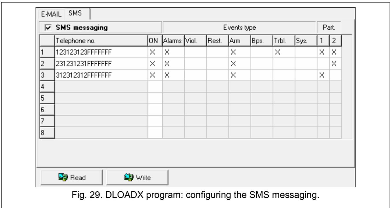
Fig. 29. DLOADX program: configuring the SMS messaging.
