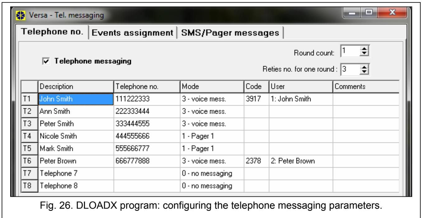
Fig. 26. DLOADX program: configuring the telephone messaging parameters.
